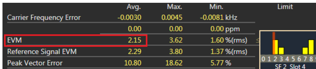
Figure 3.1.22-2 Example of Measurement Result when Test Parameter is TX3 - EVM with Exclusion Period (QPSK) (MT8821C)
